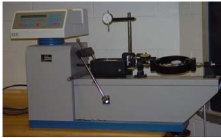
Figure 7 ASTM standard direct shear box for small dimensional granular material
